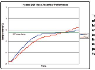
The thaw performance of a heated DEF assembly. The thaw performance and final hose assembly lengths are limited only by the maximum available power of the dosing system, Parker said.
