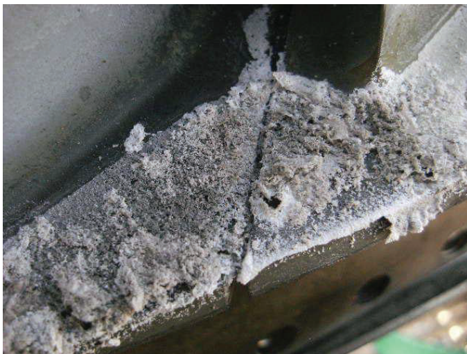
Figure 3. Inadequate gas turbine air intake filtration – sodium sulfate ( \text{Na}_2\text{SO}_4 ) buildup on power turbine blades and vanes.
